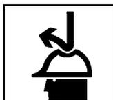
**CAUTION!** The slug is ejected at the end of the cut. Do not aim cutter or arbor so that ejected slug may hit someone around, or below you.
